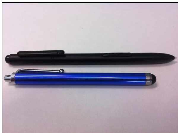
Figure 1. Comparison of Styluses: Active (top) vs. Passive (bottom)
