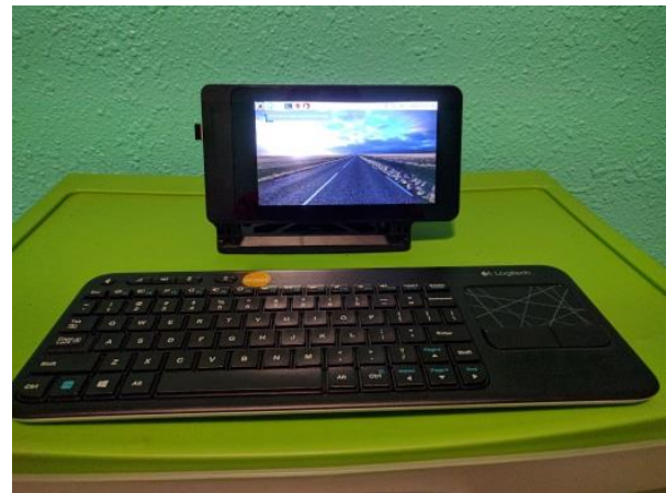
Illustration 1: Raspberry Pi 3 configured as a portable computer with a 7-inch touch screen and portable wireless keyboard.
