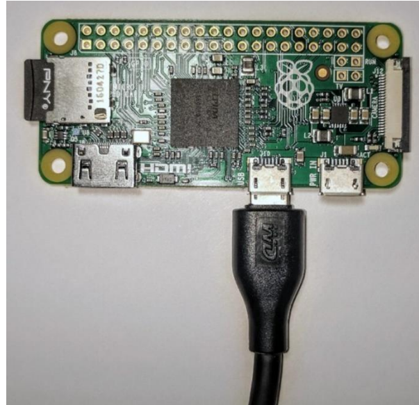
Illustration 2: Proper connection of microUSB cable when connecting to a laptop.
