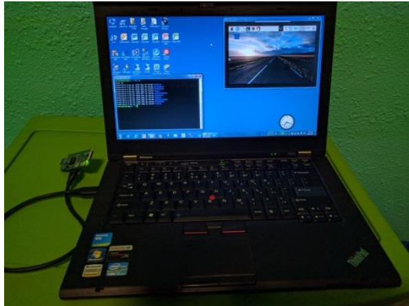
Illustration 3: Raspberry Pi Zero connected to a Windows 7 laptop with a single USB cable for power and communication. Shown with PuTTY and VNC sessions open.
